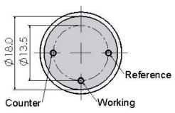
All dimensions are in millimeters. All tolerances are ±0.2mm.
